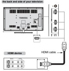
To view the HDMI device video, press O to select HDMI 1, HDMI 2, HDMI 3 or HDMI 4 mode.
